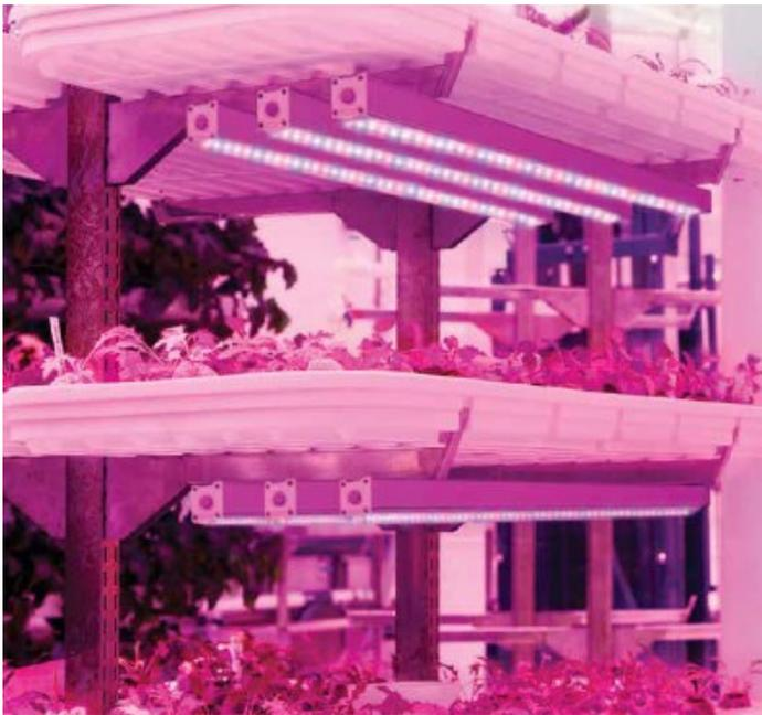
HortiLED MULTI is a small fixture that offers big energy savings, allowing for maximum space utilization and system efficacies as high as 2.5  $\mu\text{mol}/\text{J}$ .
